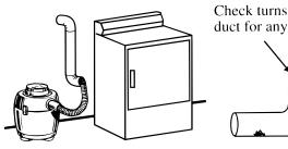
Check turns in the exhaust duct for any collected lint.
